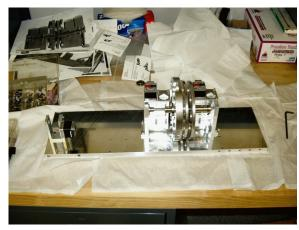
Optics bench with a few of the mechanical components mounted. Entrance aperture wheel mount is at left. Half waveplate, Wollaston and Filter wheels and the common shaft they ride on are shown. The optics mounts are not shown.
