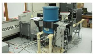
Assembled MMTPol, with the electronic boxes mounted on the side.
