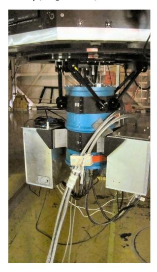
MMTPol mounted on the telescope. Note the hexapod mount and the He compressor lines. The dichroic lies above the dewar inside the mounting plate. You can just see the three micrometers that adjust its tilt hanging down from the plate.
