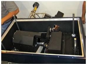
**Figure 6.** LMIRCam test fit in the NIL/NOMIC dewar. The 10 micron nuller sits below LMIRCam in this image. They are side-by-side when mounted on the telescope. The 'top' where the beam enters is on the left, about mid-thigh.
