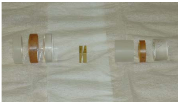
The optics for MMTPol. Sapphire, ZnSe and BaF 2 collimator on left. Rutile Wollaston prism in center. Sapphire, ZnSe and BaF 2 camera on right.
