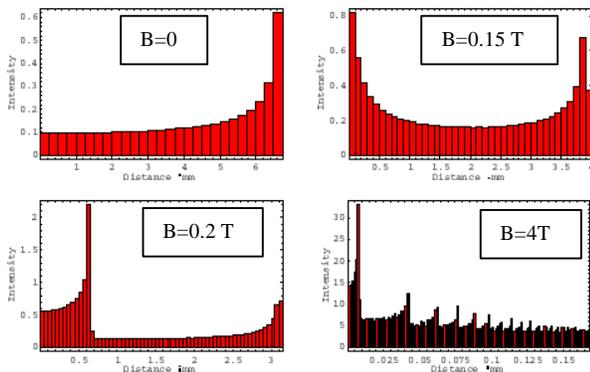
Fig. 7. Backscatter radial distributions: number of electrons as a function of distance from the impact point, for 10 keV electrons.
