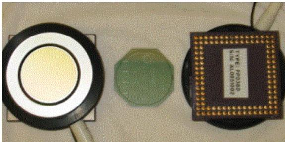
Fig. 1. The front and back of the CMS custom HPD on either side of the 19-channel hexagonal close-packed diode array which is mounted inside.
