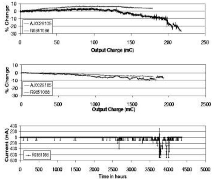
Fig. 10. Current as a function of total output charge off the anode, for 2 different pixels: top graph = CMS rate for 6 months, middle graph = Total of 6 CMS years in only 6 months. Aluminized 73-channel HPD lifetime curve is top trace; bottom trace is an early tube suffering sparking, which slowly destroys the internal vacuum. Bottom graph = high voltage supply current showing sparking problems in the early tubes.
