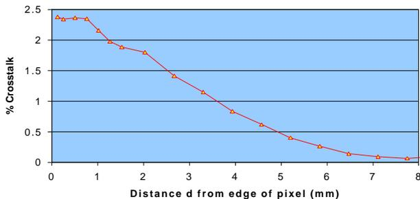
Fig. 6. Backscatter crosstalk ( $B=0$ ) with optical crosstalk ( $B=1.5$  T) subtracted for a bare silicon 19-channel HPD as a function of the position of the input light from the edge of the pixel read out. Crosstalk for fibers near the edge of the pixel compared to center.
