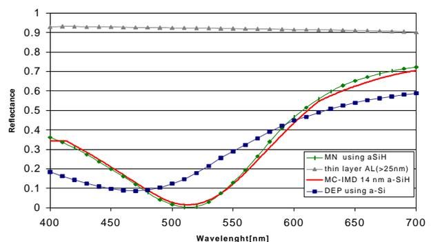
Fig. 9. 14 nm of a-Si:H deposited on aluminized glass slides matches the IMD optical modeling program. The bare aluminized slide has an approximately flat response at 92%. The DEP sputtered a-Si, with a minimum of 475 nm gives adequate reflection crosstalk reduction, but could be better optimized.
