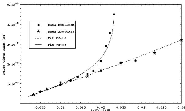
Fig. 3. Pulse width vs inverse bias voltage. Data (squares) from the earlier diodes fitted to the above model for pulse width shows that the width diverges quickly below the operating bias of  $80\text{ V}$ , whereas the new diodes (stars) with lower depletion voltage have a ‘linear’ behavior as the voltage is decreased.
