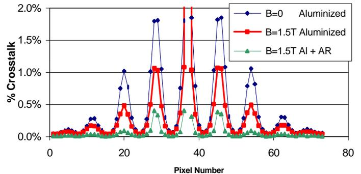
Fig. 5. The backscatter crosstalk across an entire aluminized 73-channel tube ( $B=0$ ) compared to the remaining optical reflection crosstalk once the field is turned on. The lowest crosstalk is for the tube with an anti-reflective coating over the aluminized layer.
