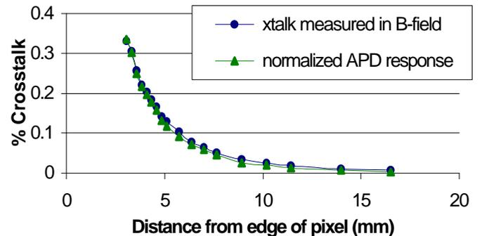
Fig. 8. Radial distribution of the optical reflection crosstalk: Circles represent the same procedure used for Fig. 6, but with  $B=1.5$  T focusing the backscatter component away. Triangles are normalized measurements from direct detection of the light (using an avalanche photodiode) which makes it back through the photocathode due to reflection off the diode.
