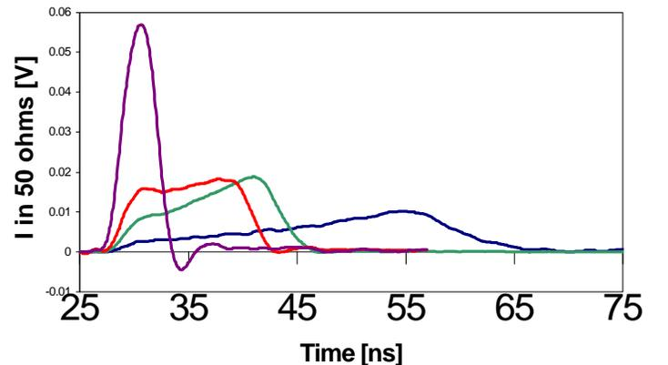
Fig. 2. Pulse shapes for (from widest to narrowest) the 300 micron and the 200 micron diodes at 80 V bias, the low-depletion, 200 micron diodes at 80 V bias and again at 500 V bias.
