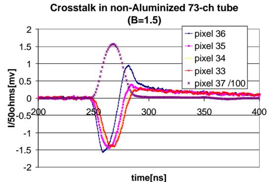
Fig. 4. AC crosstalk across a row of pixels. Light is injected into pixel 37.
