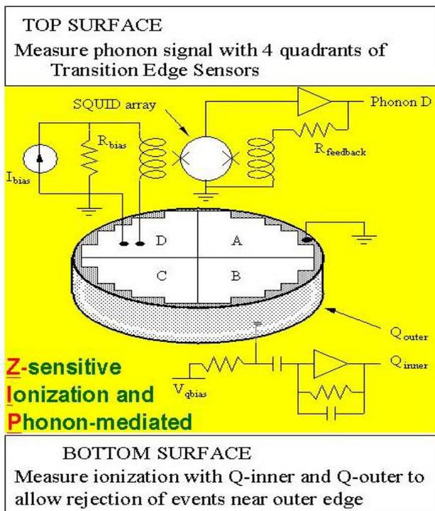
Figure 3. A diagram of the dual readout which gives CDMS such good electron recoil rejection. The athermal phonon signal is read out by TES and ionization is collected on the opposite face of the crystal.
